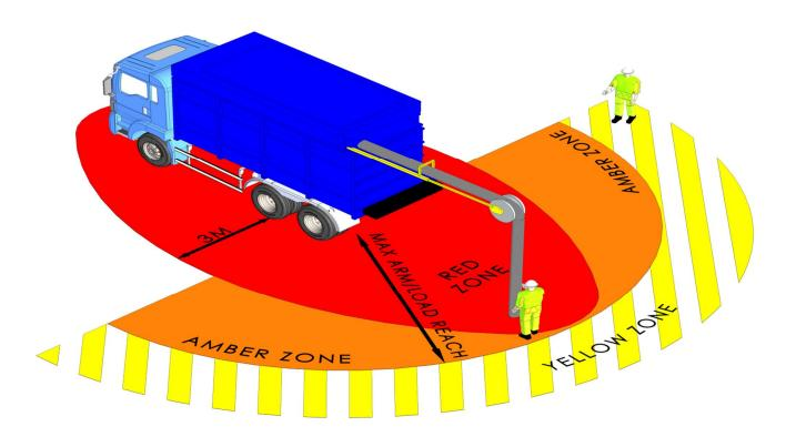
Plant Interface Zones People, vehicle and plant interface must be planned and controlled by application of the hierarchy of control (HSF-PR-0047)
